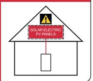
In case a string-level shutdown equipment at the PV array is used in combination with the inverter, this labeling has to be used according to NEC (Section 690.12), CEC (64-218).
