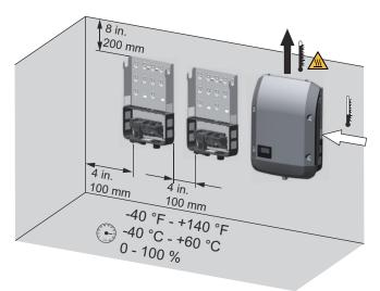
Only install on a solid, non-flammable surface
