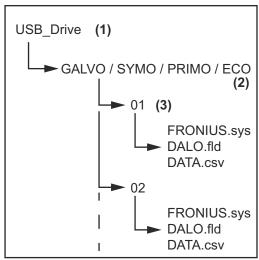
Data structure on the USB thumb drive
