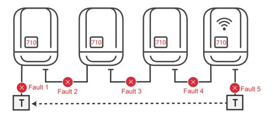
Faults occur at the beginning and end of the Solar Net ring or between the connected inverters — the primary inverter stops sending the signal, and secondary inverters switch off with status 710.
