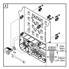
Attaching the mounting bracket to a metal carrier
