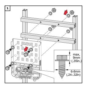
Do not warp or deform the mounting bracket **Notice!** When attaching the mounting bracket to the wall or to a column, make sure that the mounting bracket is not warped or deformed.
