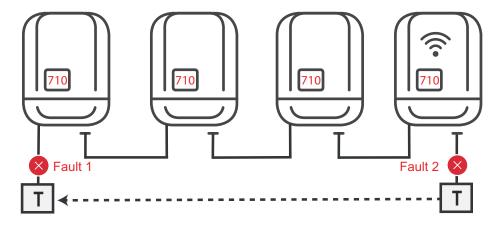
Faults occur at the beginning and end of the Solar Net ring — the primary inverter stops sending the signal, and secondary inverters switch off with status 710.
