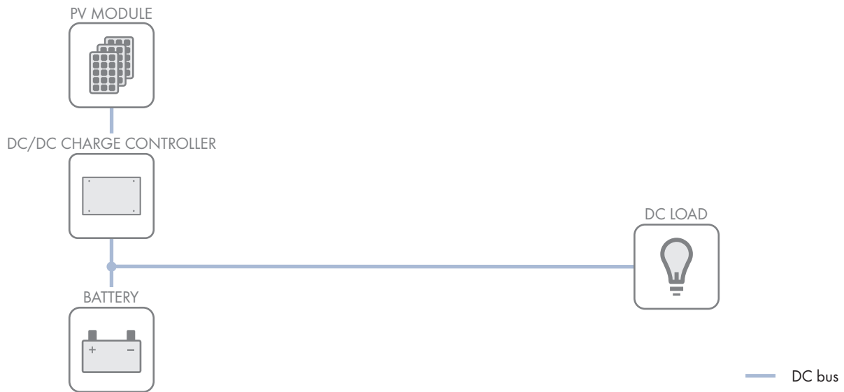
Figure 2: Example of a DC coupled system
