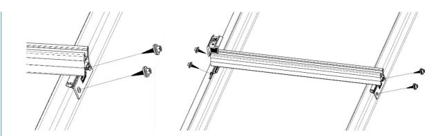
Screws must not spin! Screw on until the screw sealing ring is lightly compressed.
