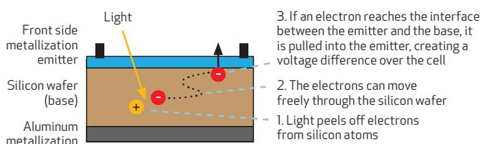
Different wavelengths of light generate electrons at different levels of the cell structure, shorter wavelengths (blue light) will generate more electrons near the front of the cell, compared to longer wavelengths (red light) which will generate electrons at the back of the cell or even pass through the wafer without generating current.
