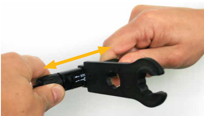
Fig. 6: Disconnecting an MC4 type connector with tool (Multi-Contact or Hosiden)
