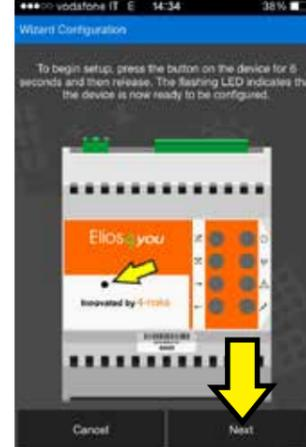
1. Hold down the configuration button (on the Elios4you transmitter) for 6 seconds, when released the LEDs will begin to flash in a clockwise sequence
