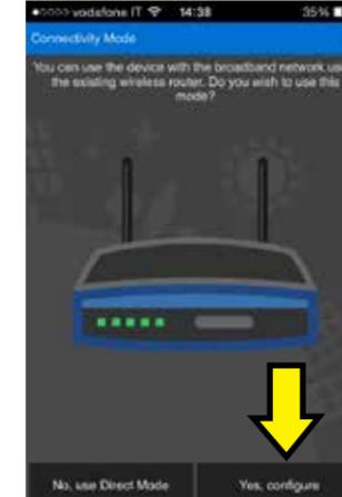
1. If you wish to connect the Elios4you transmitter to your Wi-Fi router, select "Yes, set up". Selecting "No, proceed with current settings" skip to Parameter Settings. Continue.
