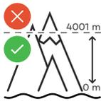
The inverter must not be installed or operated at more than 4 000 m above sea level.
