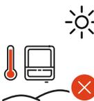
Do not expose the inverter to direct sunlight in order to keep inverter heating as low as possible.
