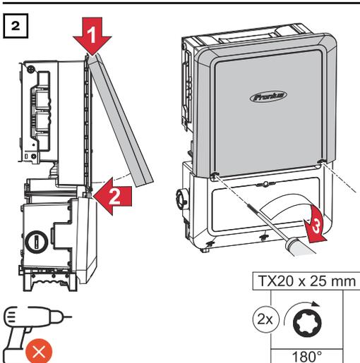
Clip the housing cover into the inverter from above. Press on the lower part of the housing cover and tighten the two screws by rotating them 180° to the right using a screwdriver (TX20).
