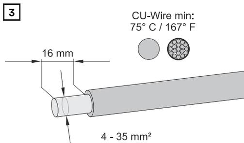
Strip the insulation of the single conductors by 16 mm. Select the cable cross-section in accordance with the instructions in [Permitted cables for the electrical grid connection](#) from page 33.
