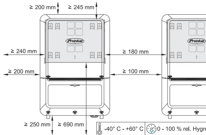
Only install on a solid, non-flammable surface.
