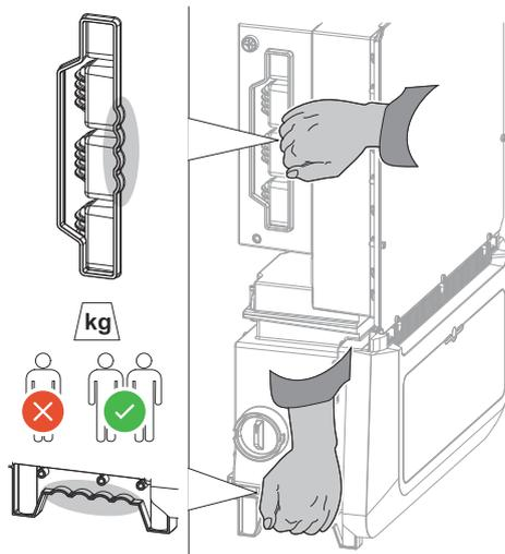
There are integrated grips on the side of the inverter which facilitate lifting/ attaching.
