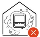
The inverter is designed to be dust-proof (IP 66). In areas of high dust accumulation, dust deposits may collect on the cooling surfaces, and thus impair the thermal performance. In this case, cleaning is required regularly. We therefore recommend not installing the inverter in areas and environments with high dust accumulation.
