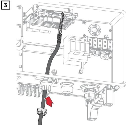
Guide the data cables first through the cable gland union nut and then through the housing opening.
