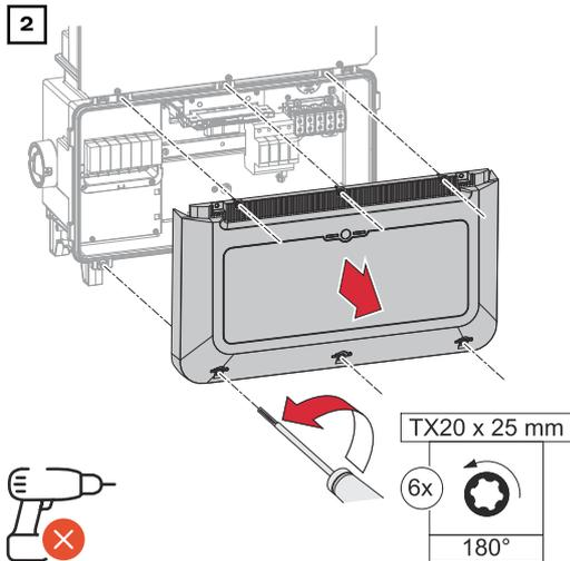
Loosen the 6 screws of the connection area cover by rotating them 180° to the left using a screwdriver (TX20). Remove the connection area cover from the device.
