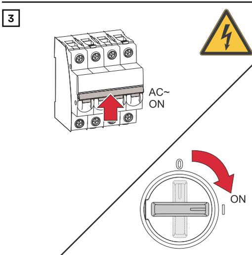
Turn the DC disconnecter to the "on" switch setting. Turn on the automatic circuit breaker.
