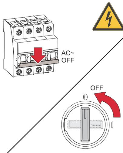
Turn off the automatic circuit breaker. Make sure that the DC disconnect is set to the "Off" switch setting.
