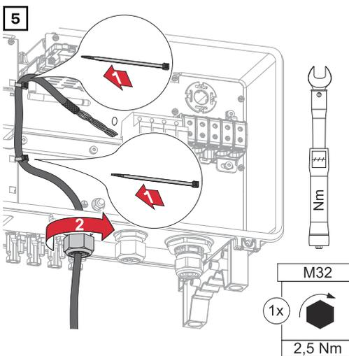
Secure the data cable to the protective cover of the DC SPD surge protection device with a cable tie. Tighten the union nut for the cable gland to a torque of min. 2.5 to max. 4 Nm.
