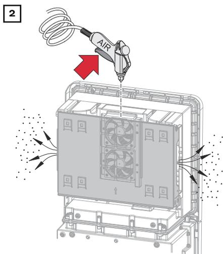
Remove any build-up of dirt on the heat sink and fan using compressed air, a cloth, or a brush.
