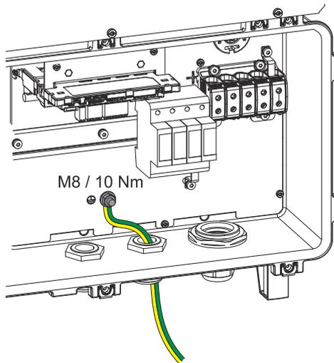
The ground electrode bolt  $\oplus$  allows additional components to be grounded, such as:
