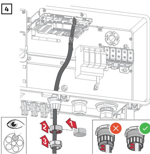
Insert the sealing ring between the union nut and the housing opening. Press the data cables into the seal's cable guide. Then press in the seal until it reaches the underside of the cable gland.
