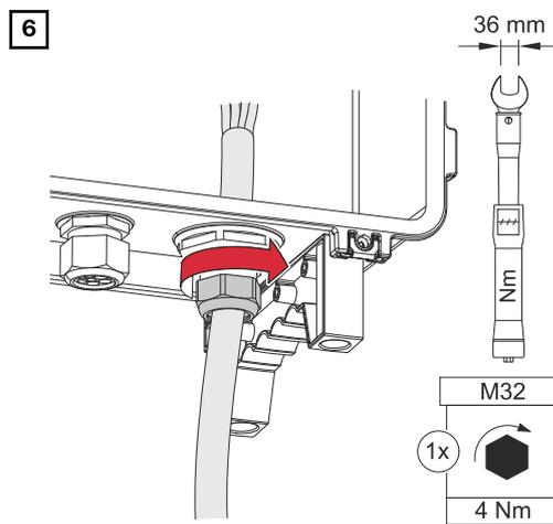
Fasten the union nut of the cable gland with a torque of 4 Nm.
