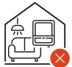
During certain operating phases the inverter may produce a slight noise. For this reason it should not be installed in an occupied living area.
