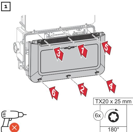
Place the cover on the connection area. Tighten six screws by rotating them 180° to the right using a screwdriver (TX20).
