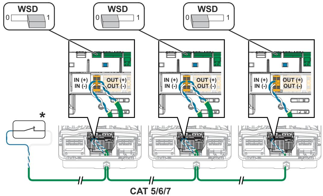
\* Floating contact of the trigger device (e.g., central grid and system protection). If several floating contacts are used in a WSD chain, these must be connected in series.
