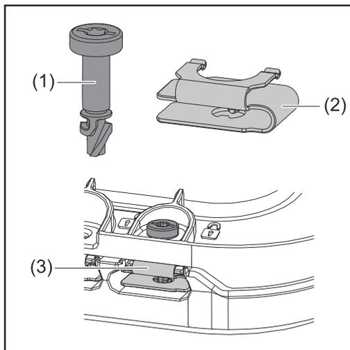
A quick-fastener system (3) is used to mount the connection area cover and front cover. The system is opened and closed with a half-rotation (180°) of the captive screw (1) into the quick-fastener spring (2).
