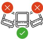
The inverter is suitable for vertical installation on a vertical wall or column.
