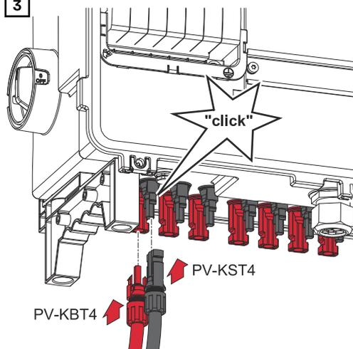
Connect PV cables from the solar modules to the MC4 plugs according to the label
