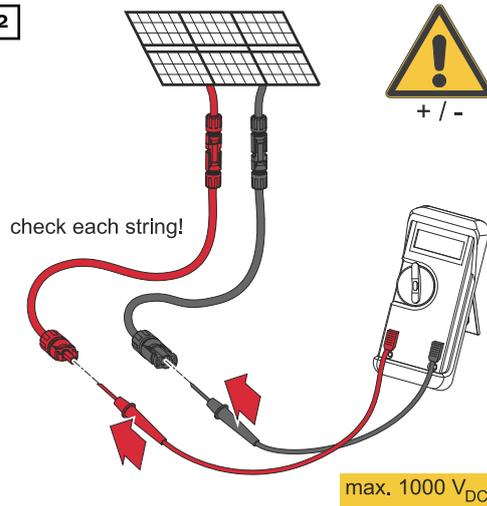
Use a suitable measuring instrument to check the voltage and polarity of the DC cabling.
