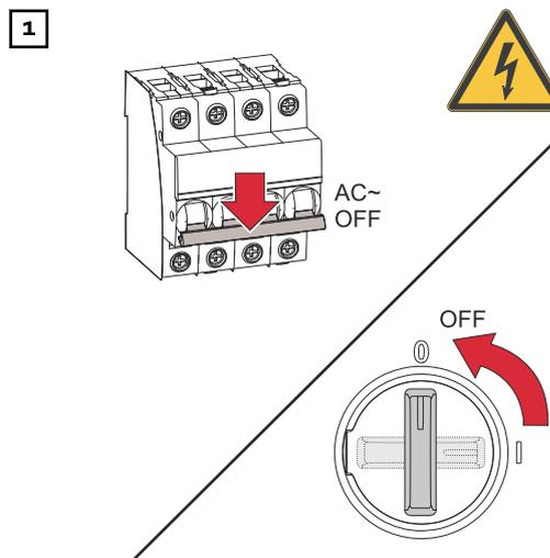
Turn off the automatic circuit breaker. Make sure that the DC disconnecter is set to the "Off" switch setting.
