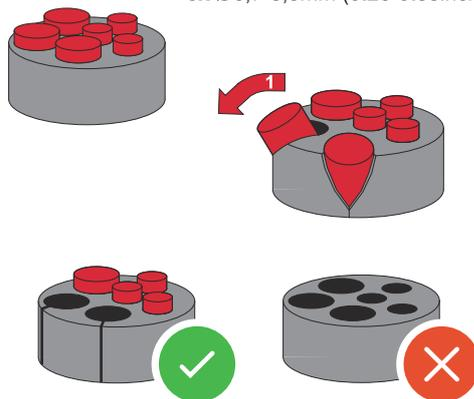
Open up the sealing ring at the location where the blanking plug is to be removed.
