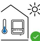
The inverter should be installed in a protected location, e.g., near the PV modules or under an overhanging roof.
