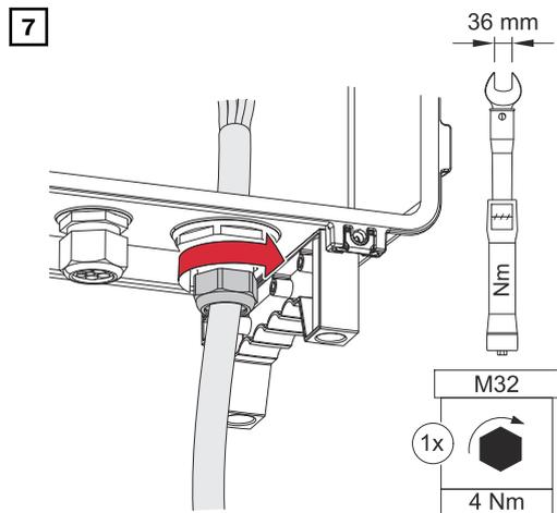
Fasten the union nut of the cable gland with a torque of 4 Nm.
