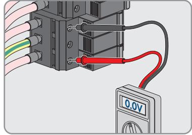
9. Ensure that no voltage is present between the positive terminal and ground as well as between the negative terminal and ground on the DC surge protection devices using a suitable measuring device. To do so, insert a test probe (maximum diameter: 2.5 mm) into the measuring points of the DC surge protection devices and hold the other one, for example, on the enclosure.
