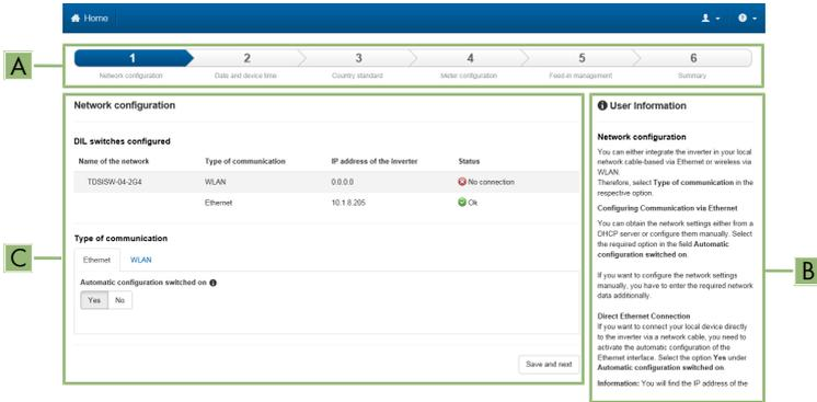
Figure 13: Layout of the installation assistant (example)
