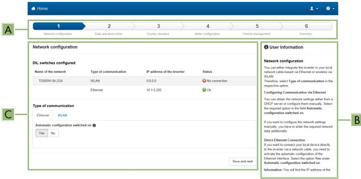
Figure 11: Layout of the installation assistant (example)
