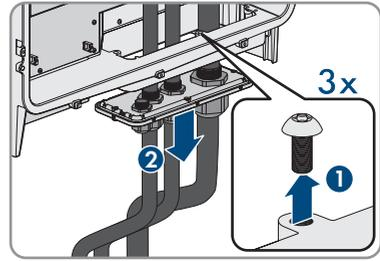
10. Position the enclosure lid and first tighten the upper-left and lower-right screws, and then the remaining screws crosswise (TX25, torque:  $6 \text{ Nm} \pm 0.3 \text{ Nm}$ ).
