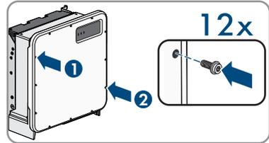
11. Screw the transport handles as far as they will go into the taps on the right- and left-hand side until they lie flush with the enclosure. When doing so, ensure that the transport handles are screwed into the taps so that they are perfectly straight. If the transport handles are not screwed in straight, this can make it more difficult or even impossible to unscrew them later on and can damage the taps to the extent that transport handles can no longer be screwed into them.
