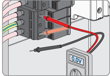
10. Ensure that there is no voltage on the AC terminal block between L1 and grounding conductor, L2 and grounding conductor, and L3 and grounding conductor using a suitable measuring device. To do so, insert the test probe (maximum diameter: 2.5 mm) into the measuring points of the respective terminal blocks.
