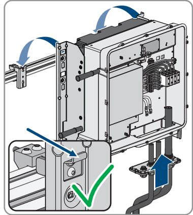
20. Align the cables according to the corresponding terminals and shorten the cables if necessary.
