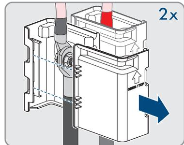
5. Remove the DC cable connection. Loosen the hex nuts (AF10) and remove the combined hexagon head screw (AF16).
