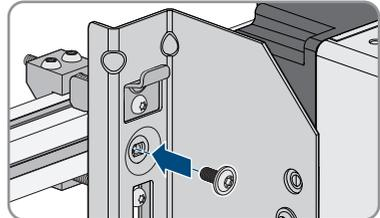
22. Remove all four transport handles from the threaded holes. If necessary, insert a screwdriver into the holes on the transport handle and use the screwdriver to remove the transport handle.
