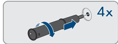
15. Insert a screwdriver into the holes in the transport handle and turn the screwdriver through 90°. This ensures that the transport handles are securely tightened.
