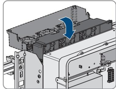
7. Press the fan bracket firmly downwards so that the locking tabs engage on the right and left.
