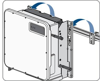
16. Remove all four transport handles from the threaded holes. If necessary, insert a screwdriver into the holes on the transport handle and use the screwdriver to remove the transport handle.
