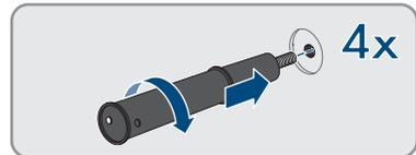
12. Insert a screwdriver into the holes in the transport handle and turn the screwdriver through  $90^\circ$ . This ensures that the transport handles are securely tightened.
