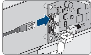
7. Ensure that the RJ45 plug is securely in place by pulling slightly on the cable.
