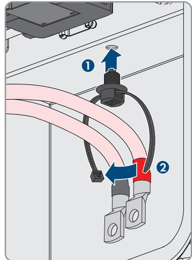
5. Mount the replacement device and make the electrical connections as described in this document. Use the connection plate and the DC protection elements against contact of the defective product.
