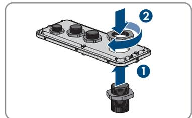
11. Lead the cables through the cable glands in the connecting plate and align the connecting plate by means of the mounting template.
