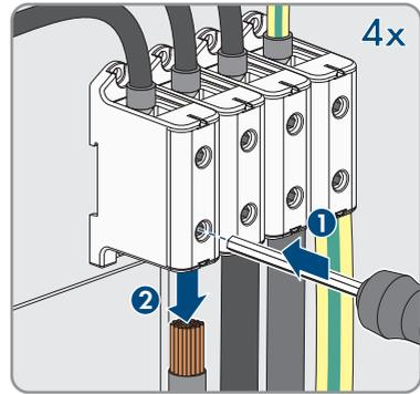
3. Remove the AC cable from the inverter.
