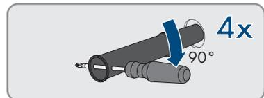
13. If the inverter is to be hooked into the mounting brackets by means of a hoist, screw the eye bolts into the threads on the top of the inverter and attach the hoist to them. The hoist must be suitable to take the weight of the inverter.
