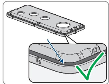
10. Attach the cable glands to the connecting plate.
