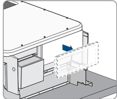
4. Secure the pre-configured DC connection cables in the defective product for transport. To do so, screw the supplied cable tie into the hole below the DC surge protection devices and place and tighten the cable tie around the DC connection cables.
