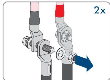
6. Remove the DC cables from the inverter.
