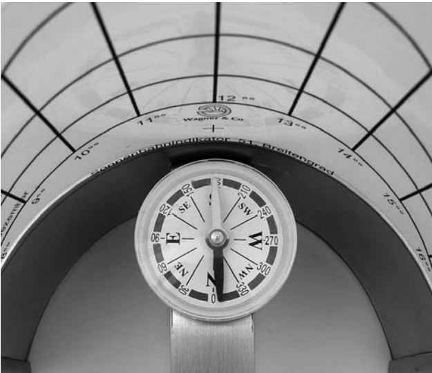
Image 4: Use the compass to align the sun path indicator South, leveling it horizontally
