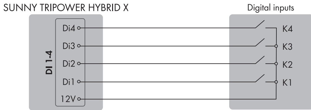
Figure 10: Connection of a remote terminal unit to the digital input DI D1-D4, Vcc of the Sunny Tripower Hybrid
